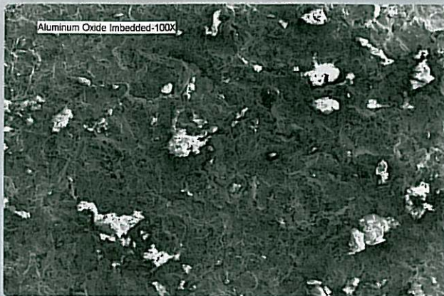
Grit blasting can leave behind fragments of its aluminum-oxide abrasive. Abrasive water-jet processing entrains abrasive materials like garnet in a high-pressure stream of water that also removes debris.
