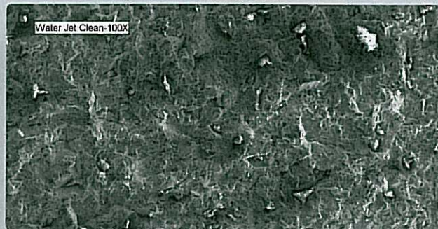
Grit blasting can leave behind fragments of its aluminum-oxide abrasive. Abrasive water-jet processing entrains abrasive materials like garnet in a high-pressure stream of water that also removes debris.
