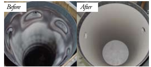
AWJ precision process cleans better, protects better and extends useful part life lowering total cost.
