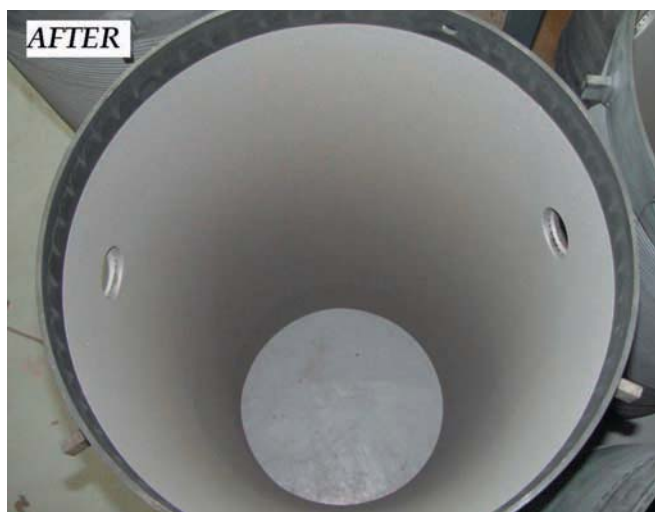
The abrasive waterjet (AWJ) process cleans coatings from aerospace and industrial gas turbine parts better than acid stripping and grit blasting, extending useful part life and lowering total cost; liner before AWJ cleaning (top); after AWJ cleaning (bottom).
