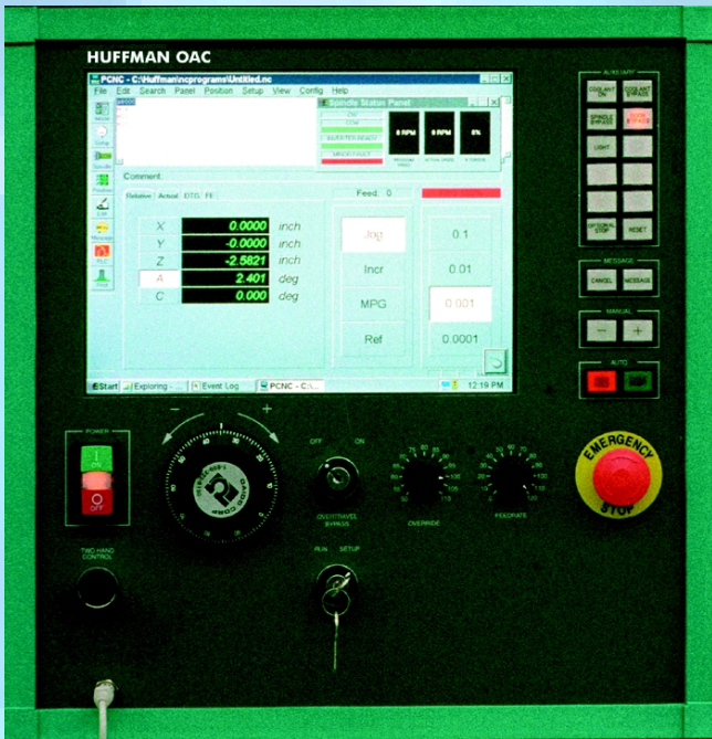
Touchscreen, LCD panel allows for quick and easy data entry and eliminates the need for a mouse.
